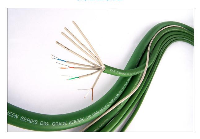
Van Damme Green Series Digi Grade cables have been specifically designed for the accurate transmission of AES/EBU digital audio signals. Low capacitance and stable characteristic impedance ensure that signals remain error and jitter free over long distances. This also makes this cable range suitable for other critical data transfer applications such as RS422, midi and timecode. Also suitable for balanced analogue audio use.
